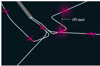
By comparison, the next-generation air traffic control system could enable incoming aircraft to continue flying the most fuel-efficient landing routes (*white*) even during heavy traffic conditions. This is because NASA's FIM technology can provide constant, automatic speed commands to pilots—no back-and-forth communication, or extra padding, needed.
