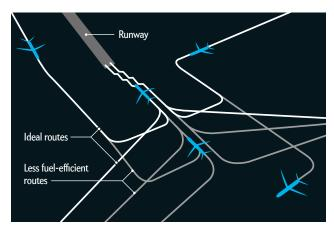
Air traffic controllers typically assign ideal routes (*white*) to each incoming aircraft. As more aircraft approach for landing, pilots are assigned longer, less fuel-efficient routes (*gray*) to ensure that a safety buffer exists between planes. The longer routes give air traffic controllers time to relay speed adjustments as necessary.
